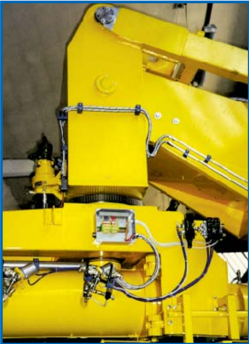
Detail shows swiveling mixer trough attached under the robust mixer arm which can be raised or lowered to suit molding box height
