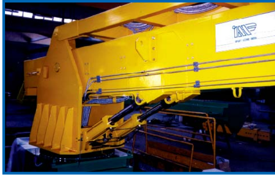
Parallelogram frame and hydraulic rams raise or lower the pivoting arm of this new IMF sand mixer enabling the mixer trough and delivery head to put sand into flasks up to 3,600 mm. high
