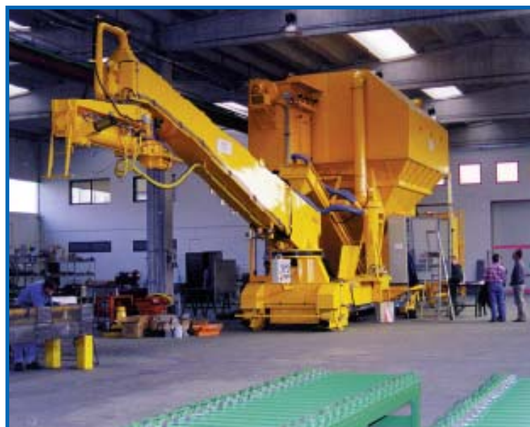
Testing of the giant mobile mixer.
