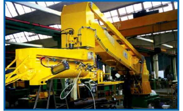
Under construction in IMF's Luino plant, a new design of elevating sand mixer which overcomes the problem of filling molding flasks of differing heights.
