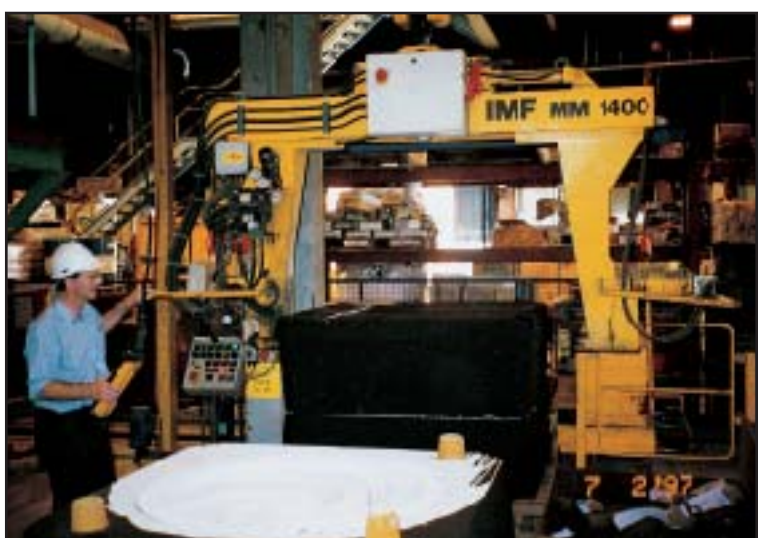
Manual mould closing station
