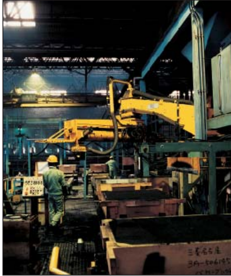
Details of the mixer during moulds filling on the Fast Loop
