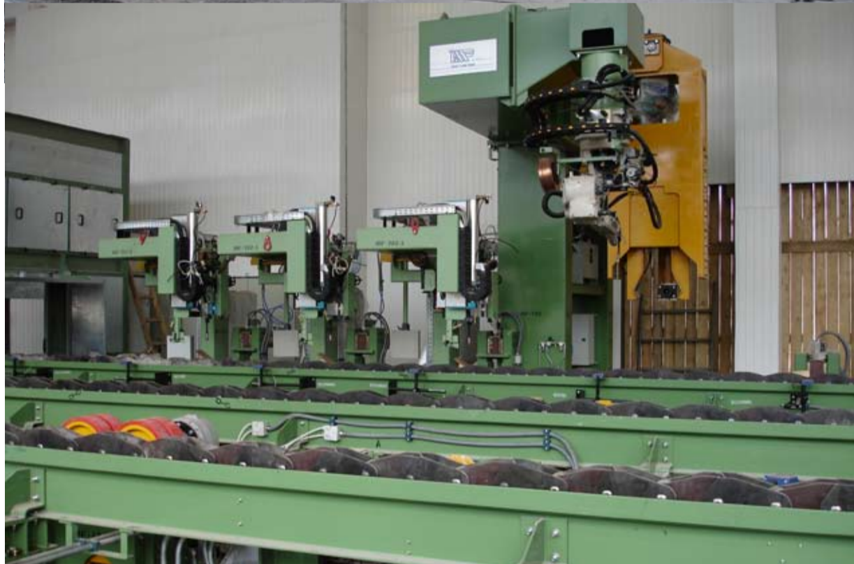
This very compact plant provides pipe machining and the automatic welding of the screw head to the pipe body by means of a robot, screw piping painting, final marking and pipe collection from the line by a manipulator.
