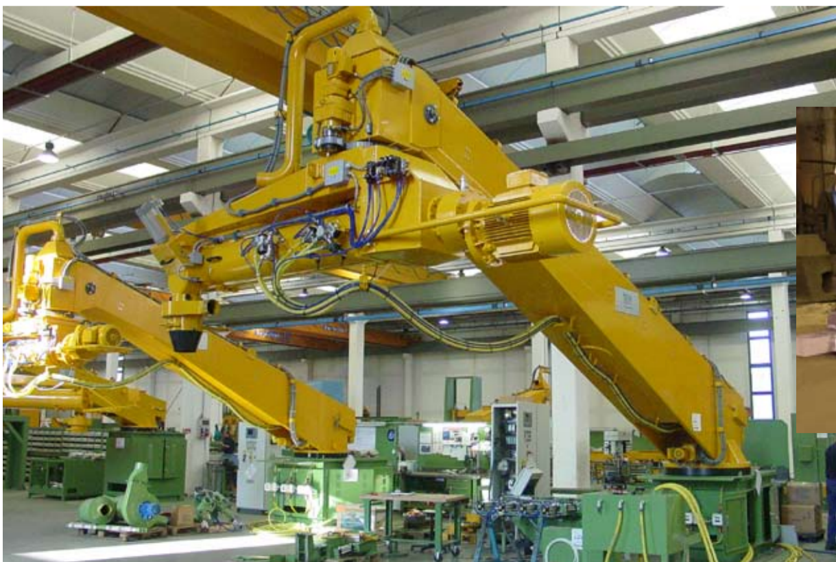
Pit moulding for these huge castings will be made with the use of two large double-arm mixers delivering 50 t/h of mixed sand each.
