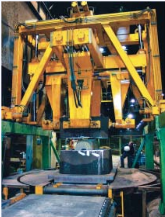
The autocloser lowers the cope on the drag previously placed on the pouring plate in the same way.
