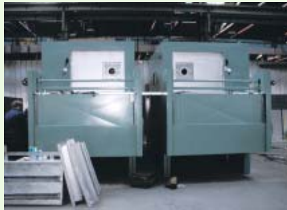
■ Gas drying tunnel
