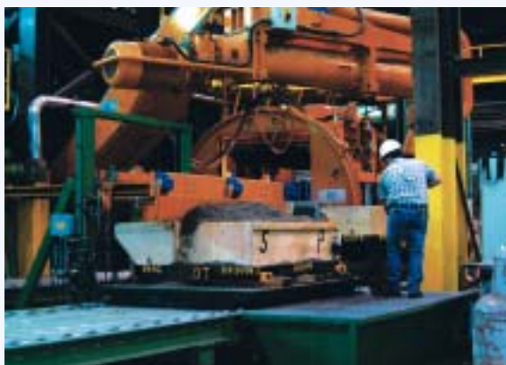
Nearly every stage of the molding loop is completely automated, including the automatic strikeoff.
