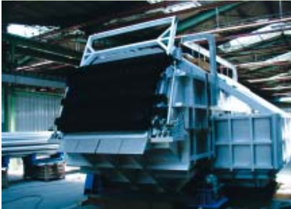
■ ALUMINIUM MELTING FURNACE
