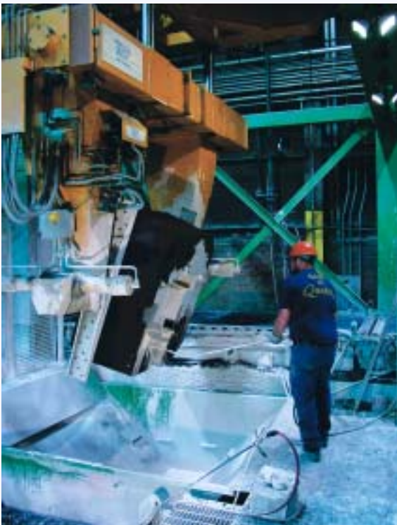
■ Each mold is automatically positioned in the center of the wash station to provide the operator with easy access. Once the wash has been applied, the mold half is automatically returned to the molding loop.
