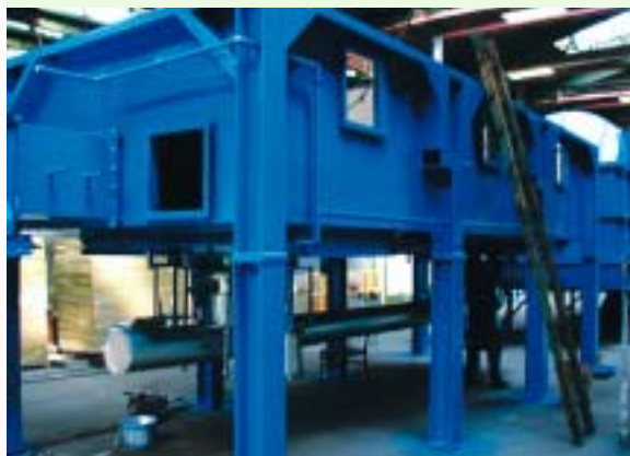
■ Afterburner for alloy wheels painting
