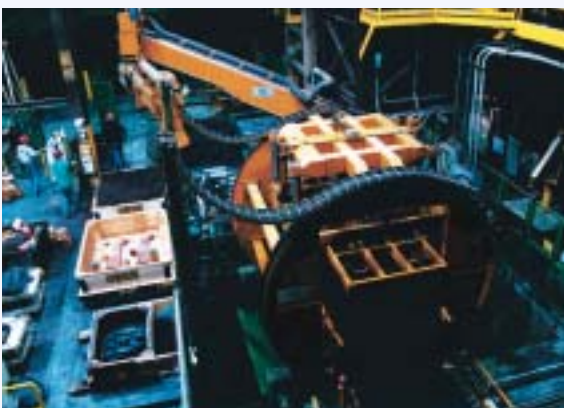
■ The rollover draw automatically strips cured mould halves from the pattern and places them on a flat belt conveyor.
